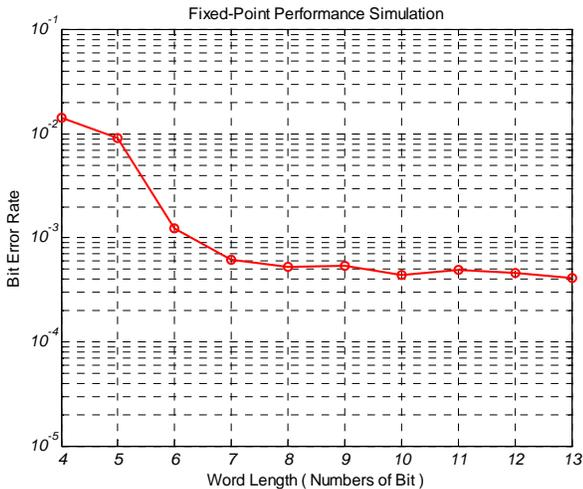
Figure 4. Word length simulation result of proposed K-best algorithm in uncoded MIMO system ( $N_r=N_t=4$ , 64QAM)
