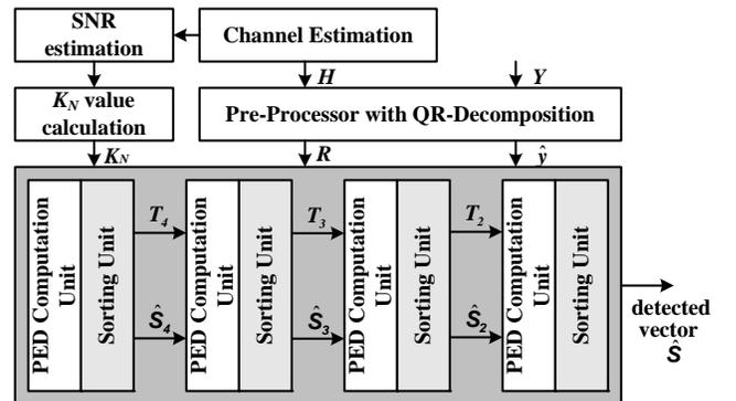
Figure 5. The flowchart of proposed K-best detector
