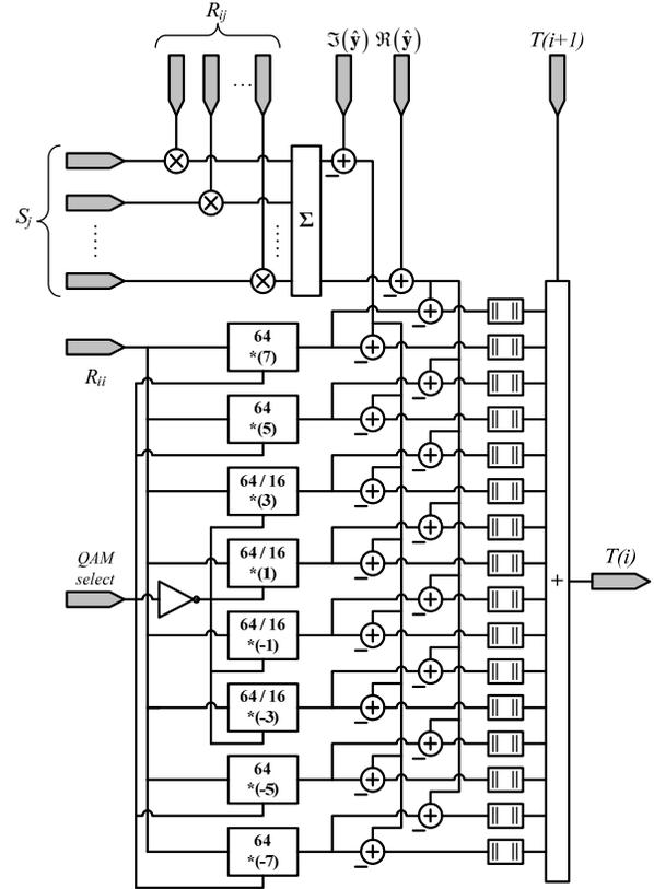
Figure 6. Architecture of PED Computation Unit
