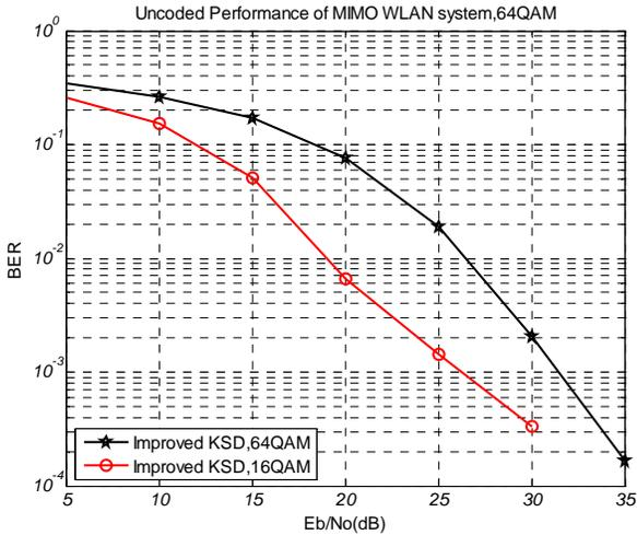
Figure 3. Simulation result of proposed K-best algorithm with 16QAM and 64QAM modulation in uncoded MIMO system ( $N_r=N_t=4$ )
