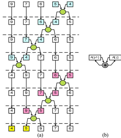
Figure 7. Architecture of Sorting Unit : (a) Data flow graph , and (b)baseline functional unit
