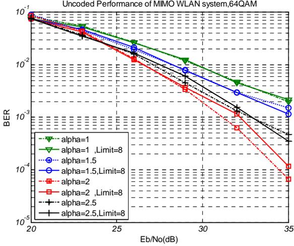
Figure 2. The uncoded BER simulation with different  $\alpha$  values form 1 to 2.5 of MIMO system ( $N_r=N_t=4$ , 64QAM)
