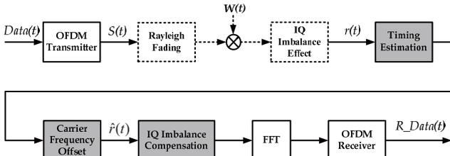
Fig. 1 System block diagram of OFDM-based basedband receiver.
