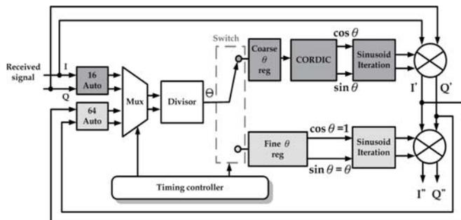
Fig. 4 Combinational circuit of fine and coarse CFO estimation.
