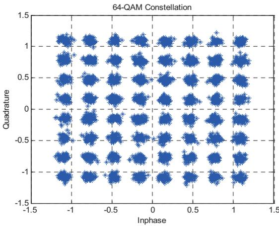
Fig. 2 64-QAM constellation compensation by CFO and IQ imbalance compensation.
