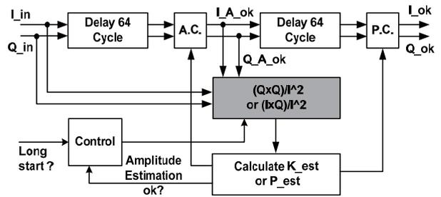
Fig. 6 The block diagram of IQ imbalance compensation circuit.
