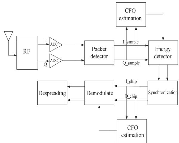
Figure 3. The Receiver block diagram.
