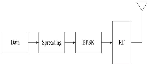
Figure 2. Block diagram of the transmitter.
