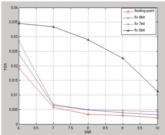
Figure 5. The simulation result of fixed point.
